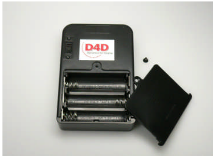
Fig.: Rear view and battery cabinet of the Voice Box
